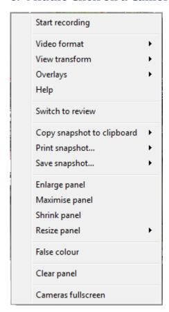
**Start recording.** If User Recording has been setup, this option will allow the user to manually trigger a recording. (An icon will appear in the top right hand corner, when a User Recording is in progress.)
