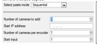
**Start IP Address** will determine the IP address of the first new camera that you are adding. The IP addresses will be incremented from here. (So make sure you have no used IP addresses in this range.)
